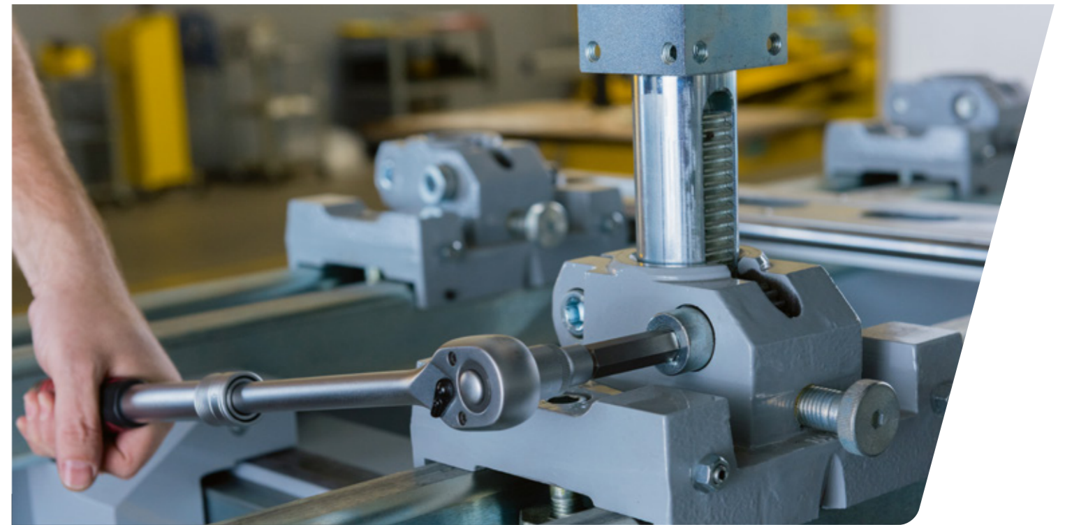
Rack system for upward thrusting and downward pulling, directly from the jig.
