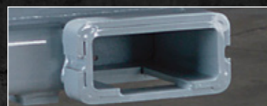
360° Pulling Tower 12 Bench mounting locations
